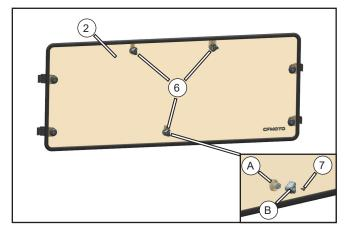
// Install the glass fastener assy (6) into the rear windshield (2) assembly position. Place the base (A) after, install the knob (B) and self-tapping φ4.8×16 screw (7) orderly. Secure them with phillips screwdriver.
