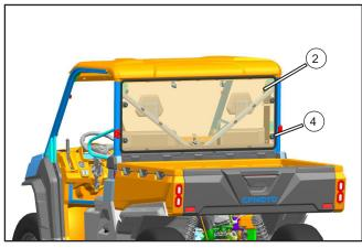
Place the rear windshield (2) into assemble position, secure four circlips (4).
