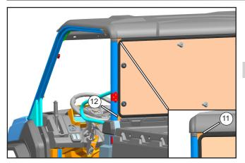
Paste the driver side upper seal foam (11) on the left upper corner of rear windshield. The driver side lower seal foam (12) on the left lower corner of rear windshield.
