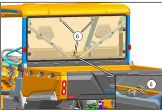
// Rotate the glass fastener assy (6) to the pic position.
