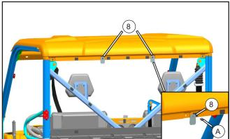
Install the rear windshield sheet mental (8) into position as shown, secure it with original bolt (A).
